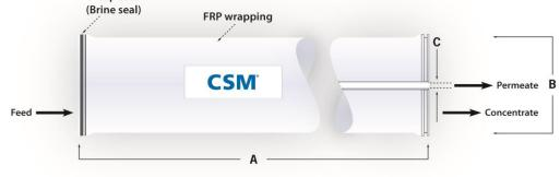
1. Each membrane element supplied with one brine seal, one interconnector (coupler) and four o-rings. 2. All RE8040 elements fit nominal 8.0 inch (201 mm) I.D. pressure vessels.
